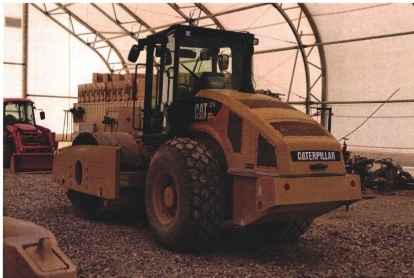
Figure 7 – Smooth drum CS74 vibratory soil compactor used for compacting south side of BAS test pad
