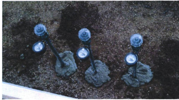
Figure 4 – Tensiometer nest at 6, 12, and 18 in. depth
