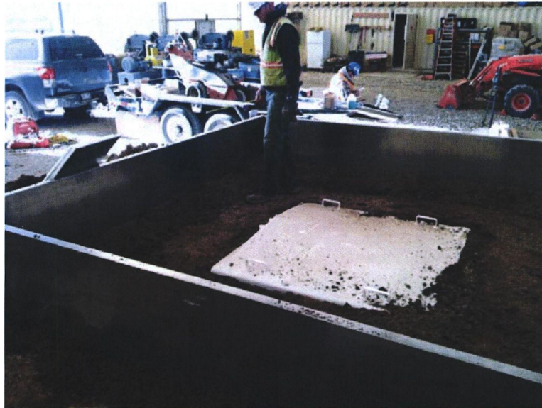
Figure 16 - SDRI with berms built on the inside around the periphery of the outer ring
