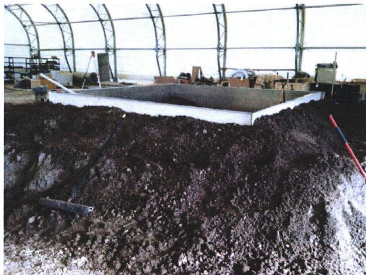
Figure 17 – SDRI with berms built on the outside around the periphery of the outer ring
